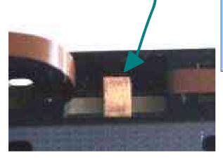
Most people have had the experience of the sound being soft or wavy, varying in volume when playing a sound cassette. The problem could be caused by the felt pressure pad that presses the tape against the tape play/record head being missing. It has fallen off. Here is a cassette tape that I have pulled some of the tape out and folded it back to show the reader the little felt pad that presses the tape against the record/play head in the machine.
